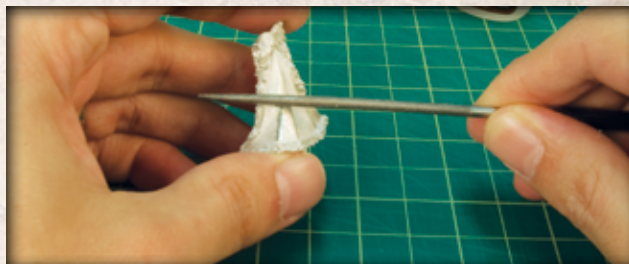
3. Filing mold lines off the cape.
