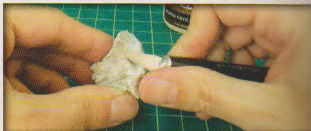
2. Using a hobby knife to scrape mold lines off the cape.
