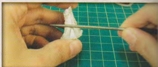
3. Filing mold lines off the cape.
