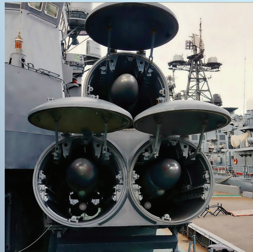
KT-120 triple cell launcher for P-120 Malakhit missiles
