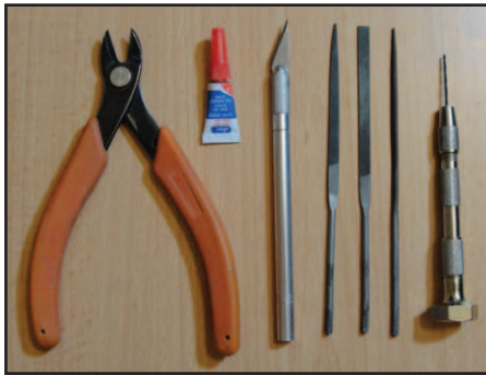
Tools and Supplies Needed (Clippers, Super Glue or Plastic Model Glue, Hobby Knife, Fine Grit Hobby Files or Sandpaper, and Hand Drill with 1/16 bit).
