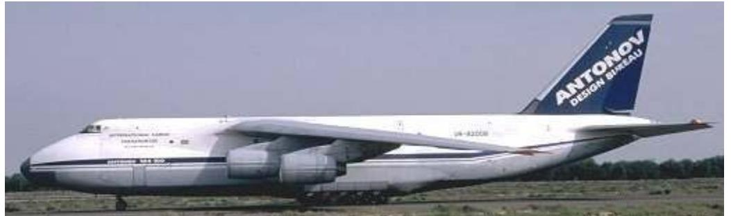
\* passenger capacity based on MaxMetal rules, various real-life sources rate it's passenger capacity from 88 to 451 passengers. The fact is that Ruslan's cargo hold is double - decked, the upper deck being fully pressurized and able to accomodate 88 troops (or passengers). The lower deck is pressurized to a much lesser degree, thus making it not advisable to carry anyone there (however, it can be done on low altitude quite safely).
