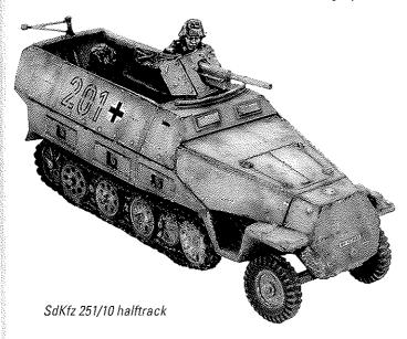
mounted MG34 machine gun, and sometimes more. Platoon commanders' vehicles carried a 37mm gun (251/10). Sometimes the anti-aircraft version (251/17) with 20mm autocannon was used as a substitute.
